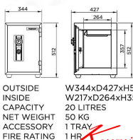
SS2DKN Outside Dimension (WxDxH)[MM.] 344 X 427 X 512 Inside Dimension (WxDxH)[MM.] 217 X 264 X 357 Net Weight 50 KG Capacity 20 Litres
